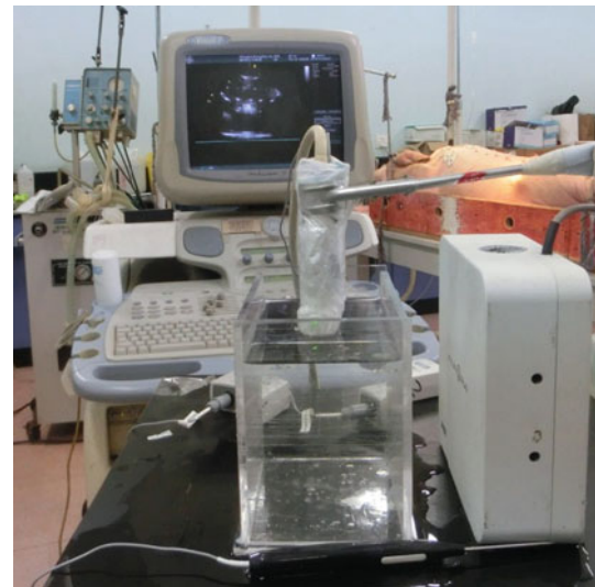
Fig. 4 The scenario of US probe calibration
